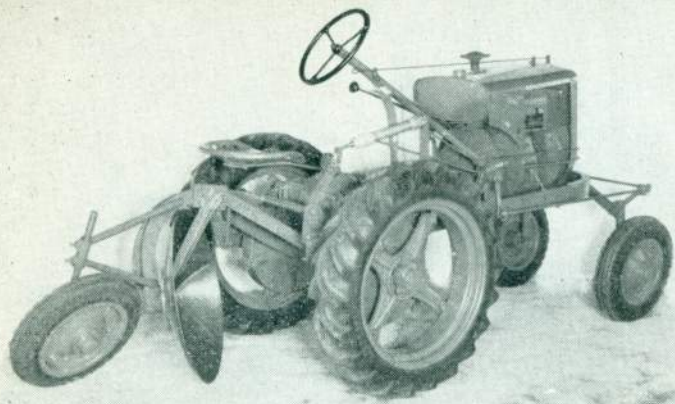
The above Model R12T SHAW DU-ALL Tractor is equipped with DP26 Disc Plow and hydraulic control. These tractors are built rugged and stand long hard service. The disc is made of heavy gauge special steel, making them very rugged and they are mounted on Timken Roller Bearings to give trouble-free long life.
