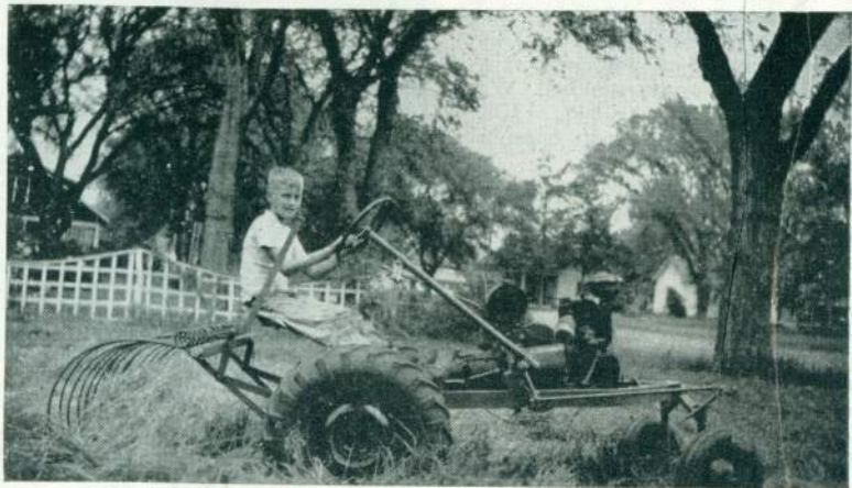
These two illustrations show the Model R6 SHAW Du-All Tractor equipped with 13OR, 5 foot Hay Rake. The rake can be quickly attached to any model SHAW Riding Tractor and is held by four bolts. When ordering, specify model of tractor so that we may supply the proper brackets. It is easily operated and a boy can manage it. Will pull much larger rakes
